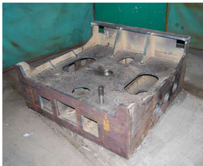
The newly constructed dragbox is seen at the Llangollen Railway Works during December 2009, before being sent away for heat treatment.
