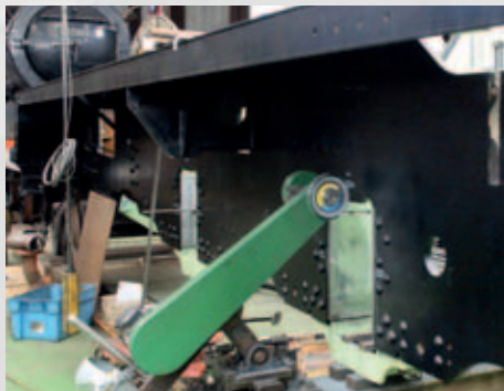
Horn guide grinding is being undertaken at Tyseley Loco Works.
