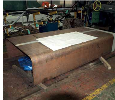
▲ The firebox crown with a copy of the original Cloughton drawings taped to the top is seen in the LNWR Workshop. PHOTO: JOHN HASTINGS-THOMPSON
