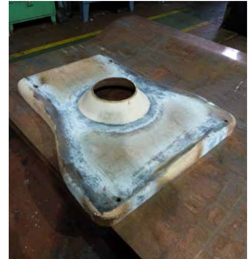
▲ The copper firebox backplate sits atop the firebox side sheets in the LNWR Workshop at Crewe. PHOTO: PETER SIKES
