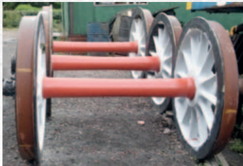
▲ The Tender Wheelsets after a coat of paint at Llangollen. PHOTO: KEVIN WEST
