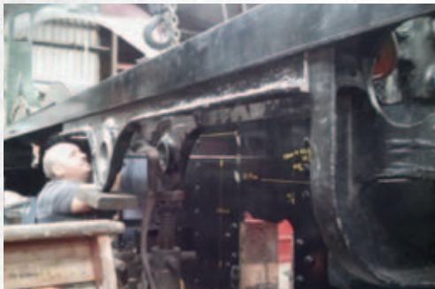
Chris Collins works on fitting the Right Hand Motion Girder. PHOTO: KEVIN WEST
