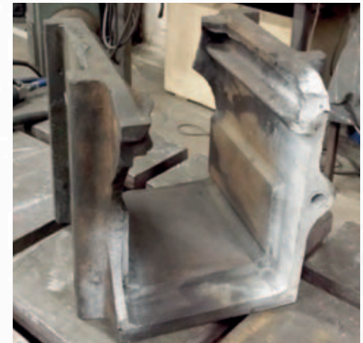
▲ Tender Axlebox before repair showing missing section.
