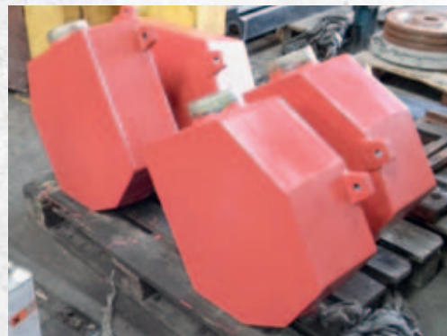
▲ The Sandboxes painted ready to fit to the chassis. PHOTO: KEVIN WEST
