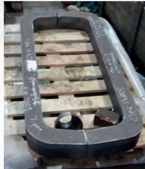
▲ Foundation Ring Corners before final machining. PHOTO - KEVIN WEST
