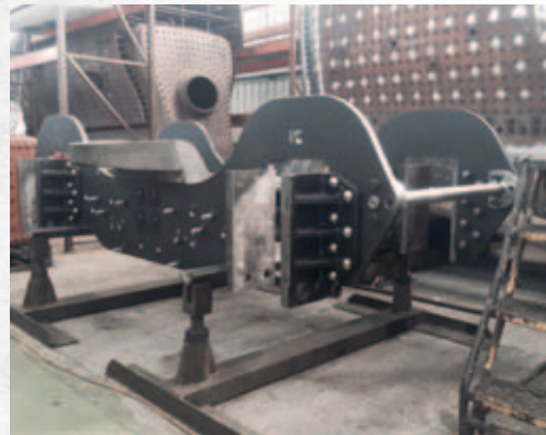
▲ The Bogie Frame Assembly under assembly at Tyseley Locomotive Works.
