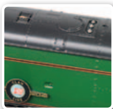
Prototypical roof safety valves - two options
