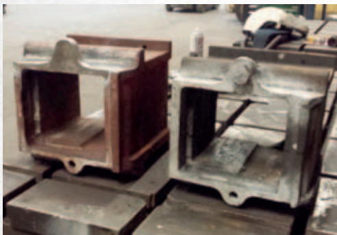
▲ Tender Axleboxes after repair. PHOTO: OAKWOOD VISUALS
