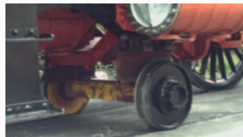
▲ The Road/Railer axle and wheels fitted to support the Unknown Warrior's front end. PHOTO: KEVIN WEST
