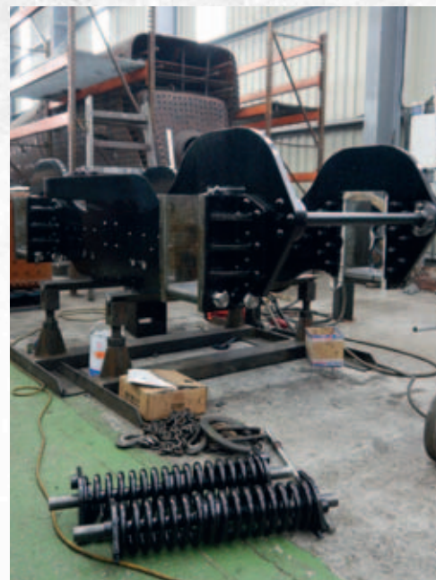
▲ The Bogie Frame under assembly at Tyseley Locomotive Works. PHOTO: ANDREW COLLINSON
