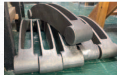
Mechanical Brake Hanger casting. PHOTO: KEVIN WEST
