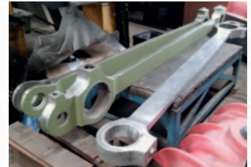
Coupling Rods showing refurbishment in progress. PHOTO: KEVIN WEST
