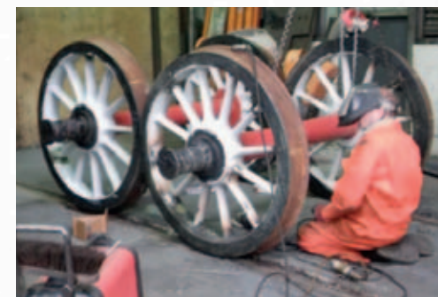
▲ Tender Wheelsets being welded at Llangollen. PHOTO: KEVIN WEST
