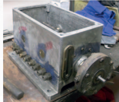
Mechanical Lubricator under overhaul. PHOTO: KEVIN WEST
