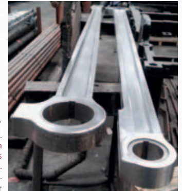
Coupling Rods showing refurbishment in progress. PHOTO: KEVIN WEST
