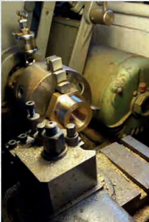
A Bulkhead fitting in the lathe ready for machining.
