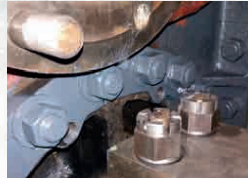
Front Outside Slidebar Fixings showing the bolts and castellated nuts.
