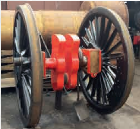
The Crank Axle Assembly with the Eccentric fitted, outside the shed at Llangollen, March 2017.
