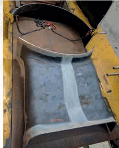
The two major parts of the Throatplate laid out at LNWR, Crewe. These parts are joined by rolled sections of plate which are welded into the gaps. Photo: Gavin Shell
