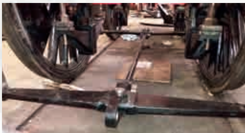
Top: The Brake Cross Shaft Bracket structure following delivery to Llangollen and being loosely assembled.
