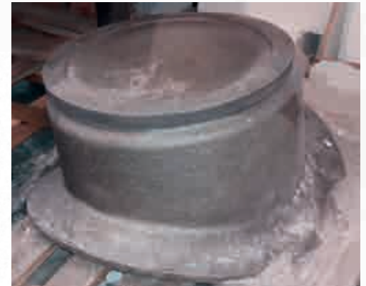
The Dome and Dome Cover castings await delivery to CMS for machining.
