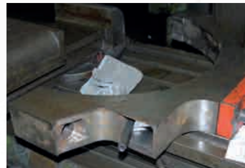
The Inside Eccentric Rod in the machine shop at Llangollen with fitting to the Front Eccentric Sheaf.
