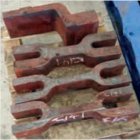
Flame Cut Blanks for the Union Links and Inside Drop Link at CMS. Two of the Union Links are for The Unknown Warrior, the third is for Jubilee 45596 Bahamas.
