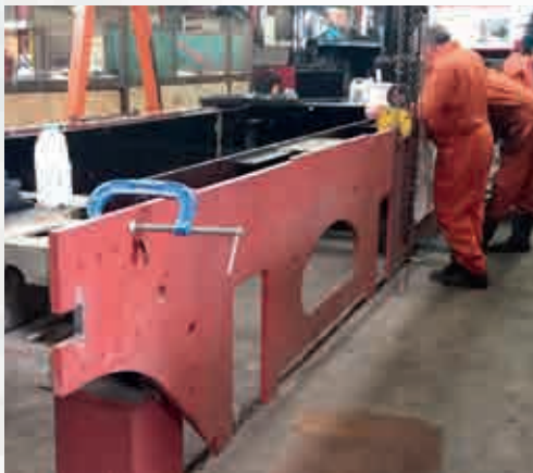
The Front Beam, drilled and in position ready for riveting.
