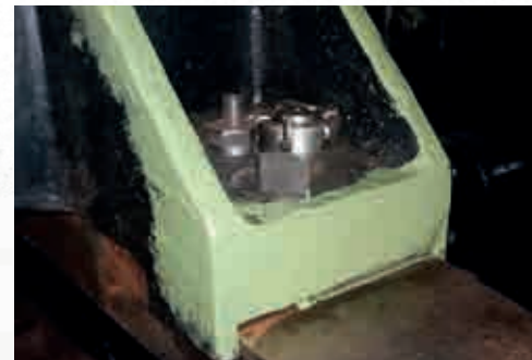
Rear Outside Slidebar Bracket showing the fixing bolts and oil pot mounting.
