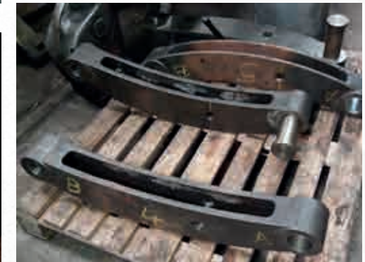
The Brake Hangers prior to being installed.
