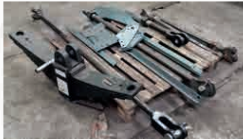
The Sanding Gear Brackets and Plates in grey undercoat along with the Trailing Brake Pull Rods and a Driving Wheel Spring.
