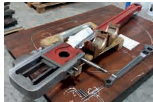
The Inside Connecting Rod assembly in the machine shop at CMS.
