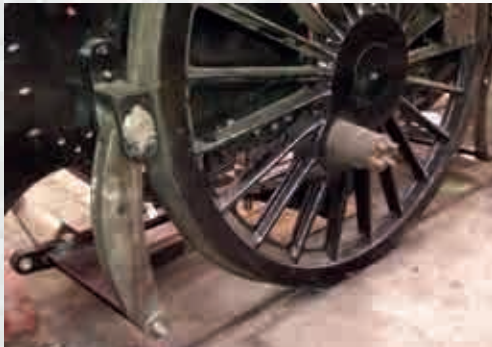
Below left: A close up view of the Brake Gear for the Middle and Rear Driving Wheels during assembly.
