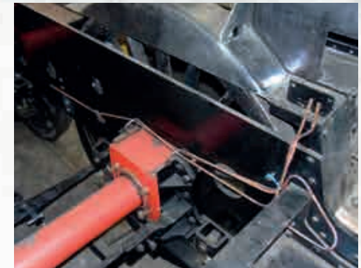
The first of the Lubrication Pipework being installed. These are for lubricating the Trailing Horn Guide Slides.
