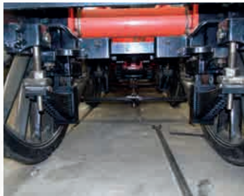
Top: The Brake Cross Shaft Bracket structure following delivery to Llangollen and being loosely assembled.
