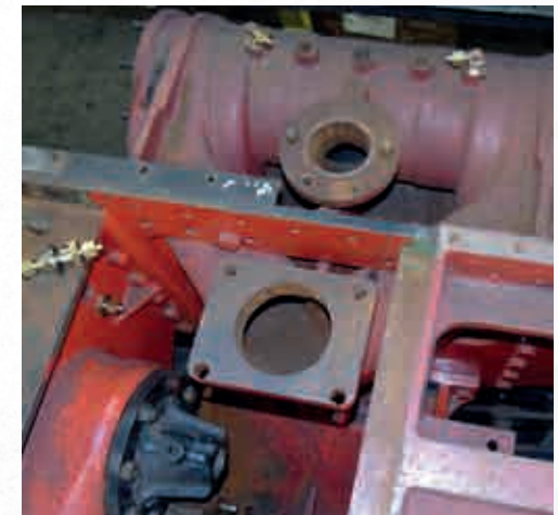
The non-return valves installed in the Valve Chest of the right cylinder and the bulkhead fittings being installed on the rear face of the Inside Cylinder.
