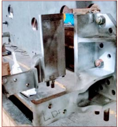
The Horn Guides for the leading axle mounted onto the left hand frame plate. PHOTO: NEIL KINSEY
