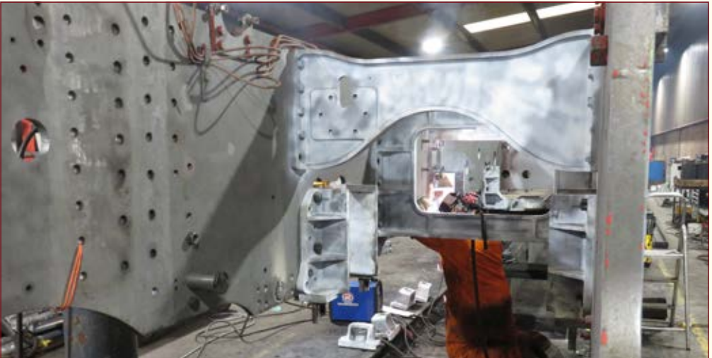
A view between the frames of 5551 at West Shed. The recently repaired Stretcher is mounted onto the rows of vertical holes visible on the left. PHOTO: KEVIN WEST
