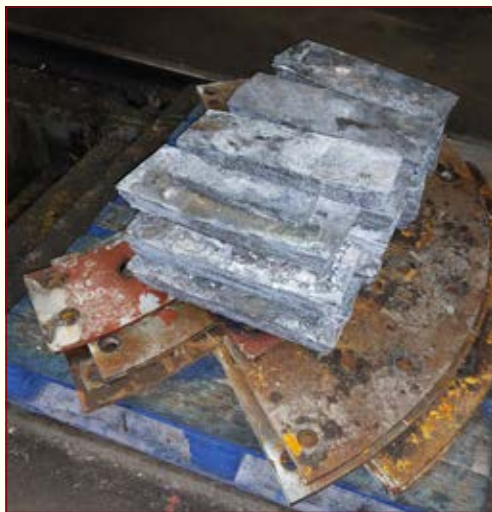
The Balance Weight Plates and balancing lead following recovery from the old Driving Wheels. PHOTO: KEVIN WEST
