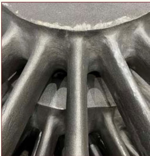
A close up view of one Driving Wheel showing the quality of the casting. PHOTO: COLIN HALL
