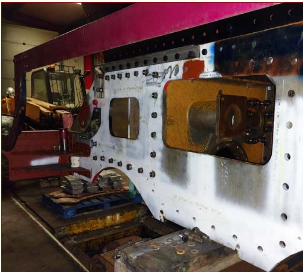
A view of the front end of 5551 showing the Inside Cylinder in position through the left hand frame plate. PHOTO: KEVIN WEST
