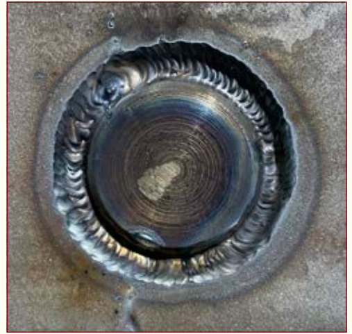
Above: Building up the ring of weld in progress and (below) a batch of holes following completion of welding, but before grinding back to a smooth surface. BOTH PHOTOS: KEITH RICHES
