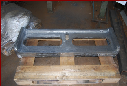
Two of the frame stretchers after being cast at the Boro Foundry
