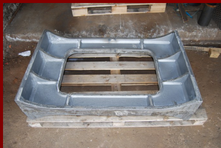
Two of the frame stretchers after being cast at the Boro Foundry
