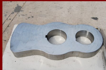
One of the driving wheel webs after machining
