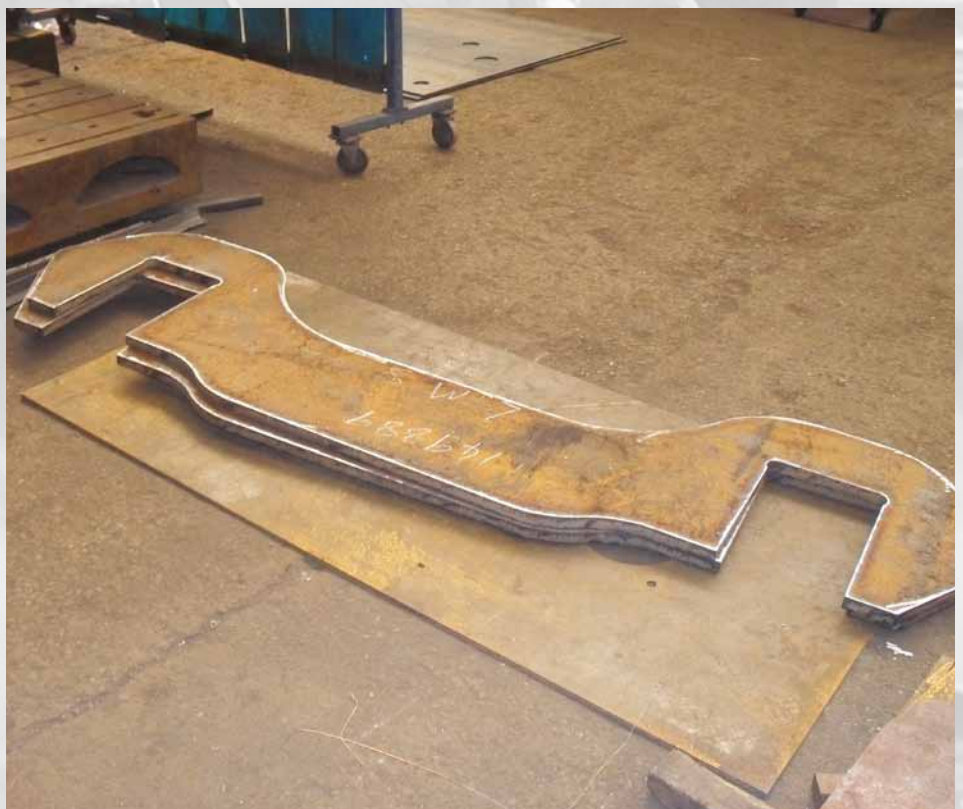
The newly cut bogie frame plates at Morgans UK Ltd, Tyseley.
