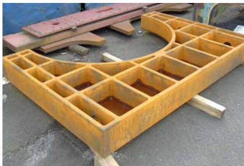
▲ The formers are negative shapes for either inside or outside of the desired shape. This view shows the back of the block that will be used to create the flange for the barrel joint in the circular cut out.
