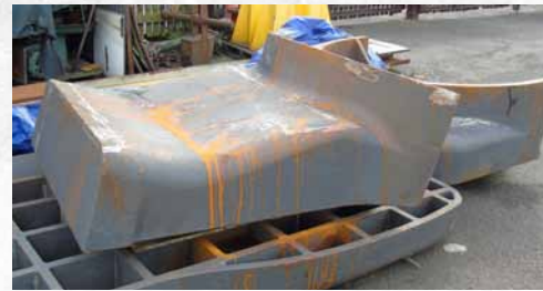
▲ This is the Inner Former for the lower section. The step will be pressed into the plate and after forming the barrel flange on the block shown above the side flanges are formed here. The top section block is to the right. The former underneath is a Doorplate for a large GWR 4-6-0.
