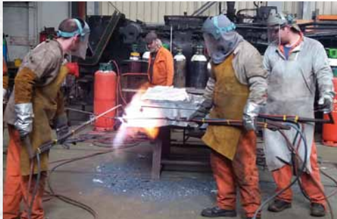
▲ The Outer Firebox Doorplate top corners being heated before the next stage to hammer it down over the former.
