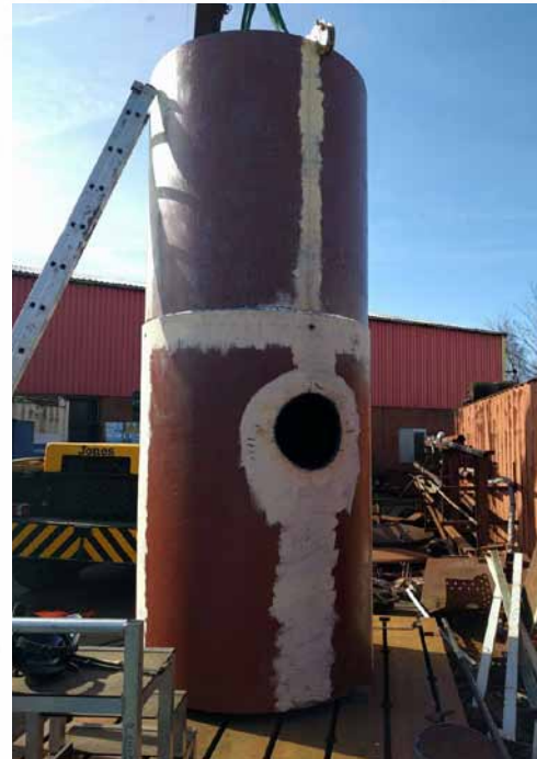
▲ Boiler barrel assembly underway at LNWR Crewe. The two barrel sections have been assembled and the dome hole cut.
