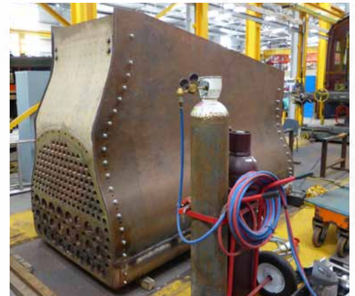
▲ Inner Firebox assembly underway at LNWR Crewe. PHOTO: GAVIN SHELL
