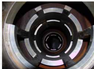
▲ Left hand Outside Valve Liners in position in the cylinder showing the positioning jig ensuring the liner is at the correct depth.
