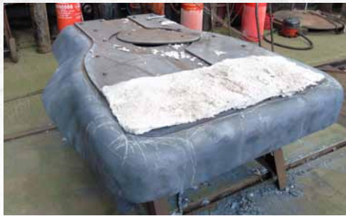
▲ This view shows the top corners have been formed with just the right hand flange waiting to be knocked down. The row of gas bottle in the background illustrates just how much is needed for the plate forming.
