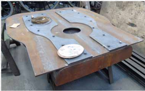
▲ The Outer Firebox Doorplate blank bolted to the former block at Tyseley Locomotive Works.
