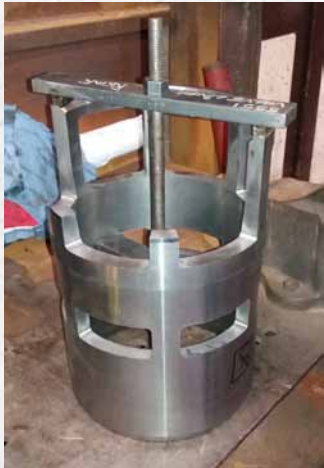
◀ One of the Valve Liners in its positioning jig, ready to be placed in the liquid nitrogen.
