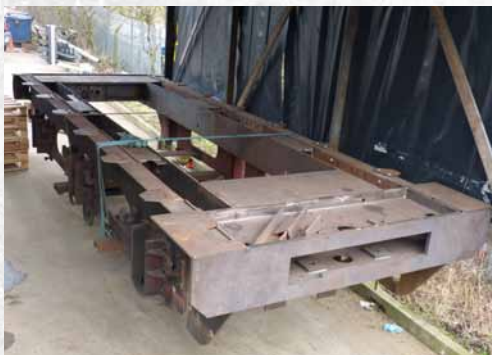
▲ The Tender Chassis following refurbishment at Rowlescourt Engineering.
