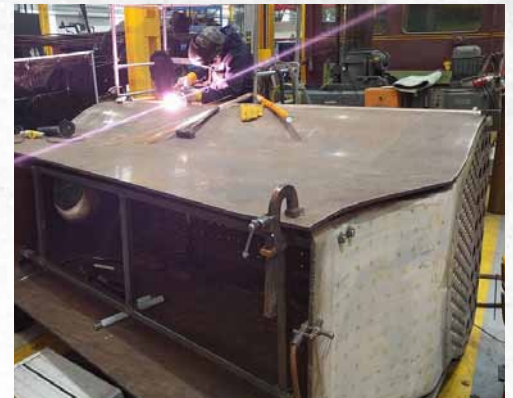
▲ Inner Firebox assembly underway at LNWR Crewe. PHOTO: GAVIN SHELL
