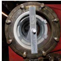
▲ Left hand Outside Valve Liners in position in the cylinder showing the positioning jig ensuring the liner is at the correct depth.
