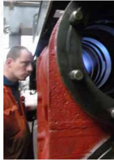
▲ Warming the right hand Outside Cylinder with a gas torch.
