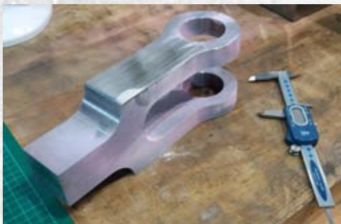
One of the Pull Rod End under manufacture at CMS Ceper, June 2016.
