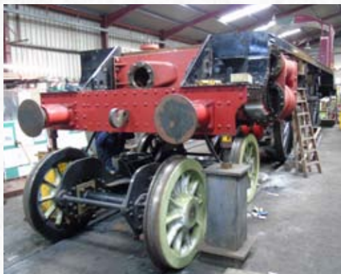
The Chassis jacked up to allow work on the frame assembly. May 2016.
