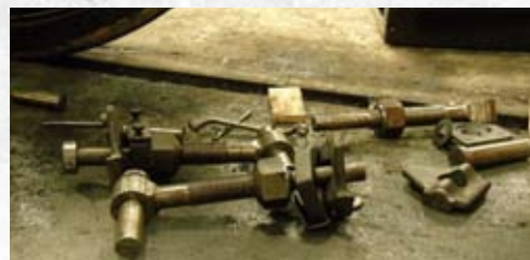
A selection of the Hangers, Pins and fittings for the Springs during the trial fitting. May 2016.
