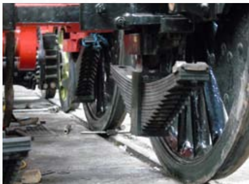
The above two images show the Main Springs during trial fitting in May.
