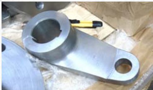
One of the Lubrication Drive Cranks. Just one part of the many parts required for the smaller systems on the locomotive, June 2016.
