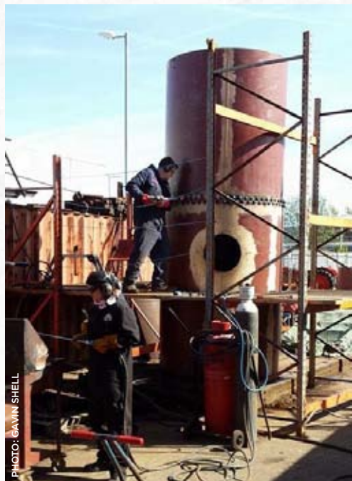
The Boiler Barrel sections being riveted at LNWR Crewe, May 2016.
