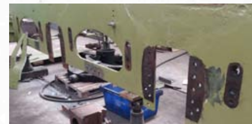
The original Frames showing the Horn Guides and Spring Hangers have been removed.
