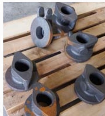
The Cylinder Relief Valve castings at CMS for machining.
