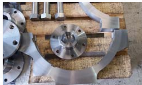
The Eccentric Sheaf Halves and a selection of other motion parts at CMS before delivery to Llangollen.
