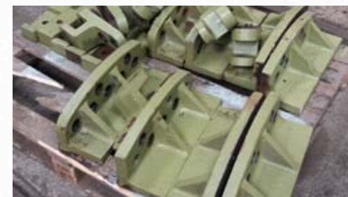
The Horn Guides and Spring Hangers removed from the original Frames.
