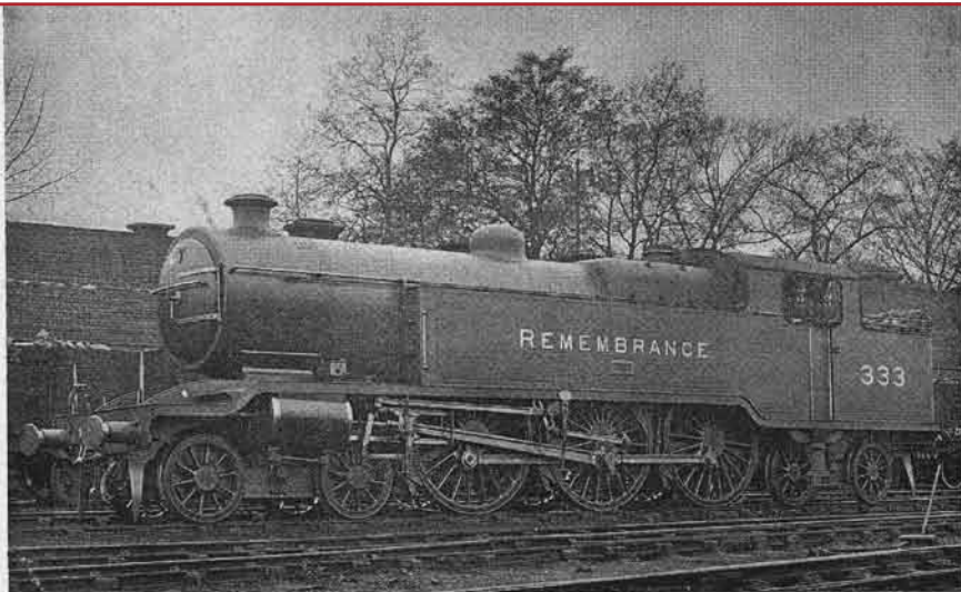
London, Brighton & South Coast Railway 4-6-4 tank engine No. 333, "Remembrance", in pre-grouping livery, as built at Brighton Works in 1922
