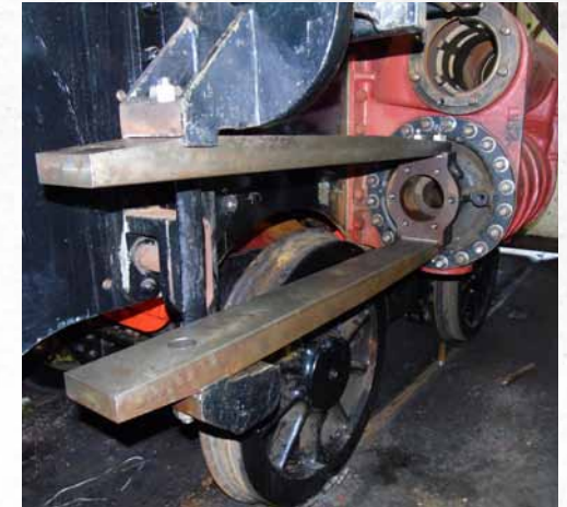
The right hand Outside Cylinder with Rear Cover in place and Slide Bars fitted.
