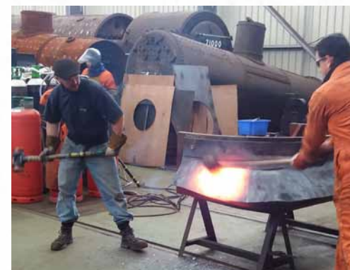
Throatplate Top 3 Alistair Meanley works on another section of the flange.
