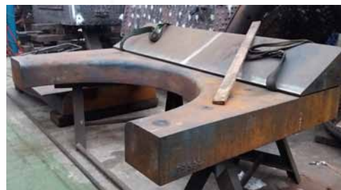
The Barrel flange former with the wedge shaped used to support the bottom section placed on top.
