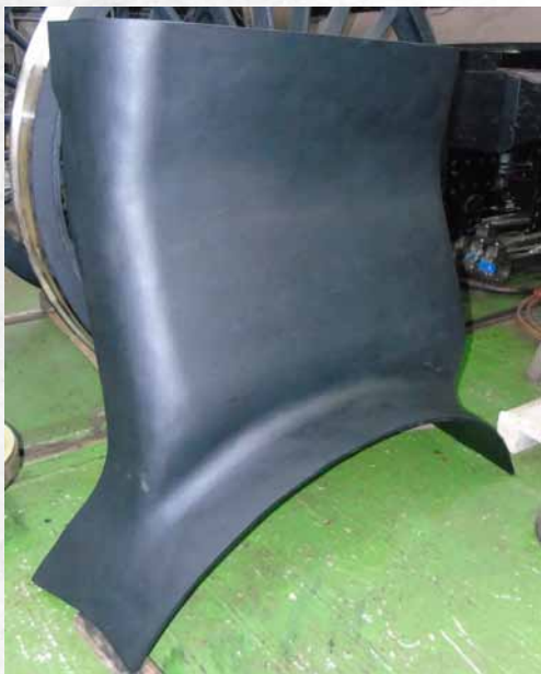
The bottom section of the Throatplate following forming at Tyseley Locomotives Works.
