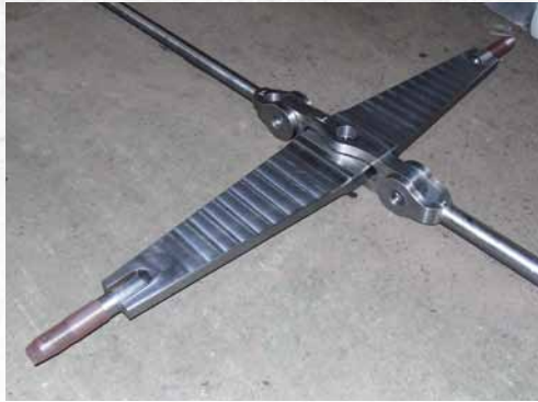
The detailed view of the Cross Beam, Bridle and Pull Rods.
