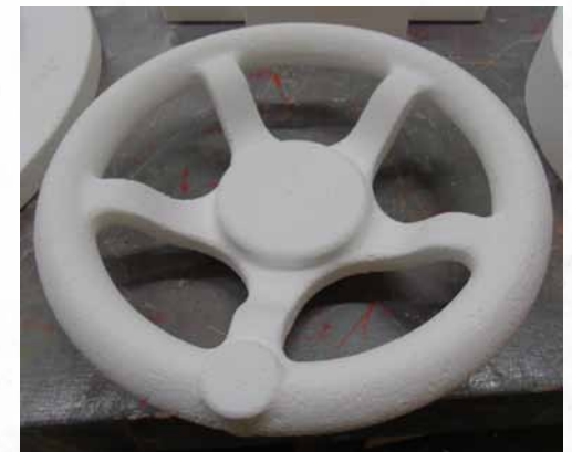
The pattern for the sculptured Reverser Wheel.
