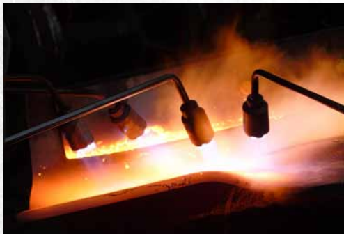
A view of a section of the Throatplate during heating before being hammered over the former. Each heating cycle takes 7 to 8 minutes to get the sheet hot enough for 30-40 seconds of forming.
