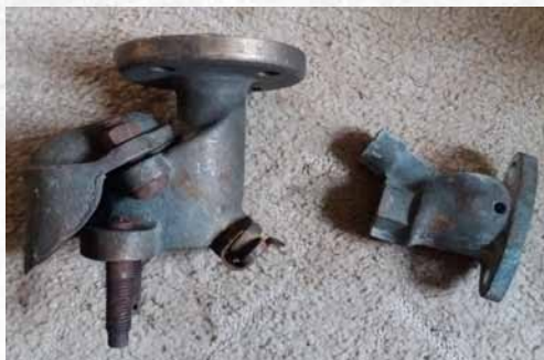
A Sand Trap and Nozzle prior to refurbishment.
