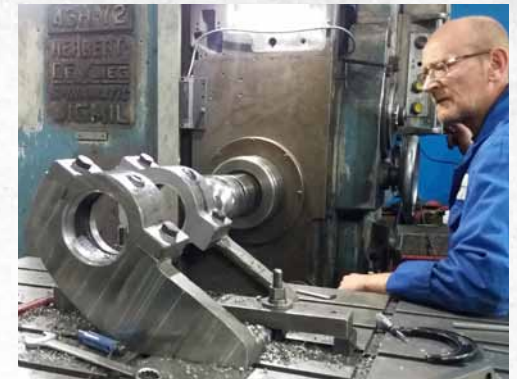
Intermediate Reverser Shaft Bracket undergoing machining at Harco Engineering.
