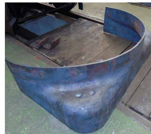
Throatplate Top 4 The finished top section of the Throatplate. The only section of plate that is in the same plane as the original sheet are the two sections in the corners where the two fixing holes have been welded.
