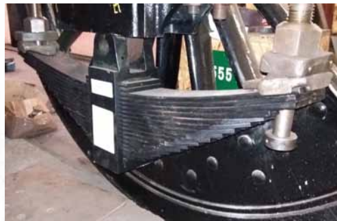
The new design Driving Wheel Spring trial fitted to the locomotive chassis.
