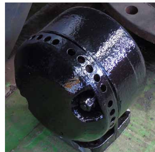
One of the Snifting Valves from Jubilee 45596 Bahamas at Tyseley Locomotive Works.
