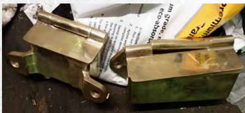
Two of the Oil Boxes following polishing
