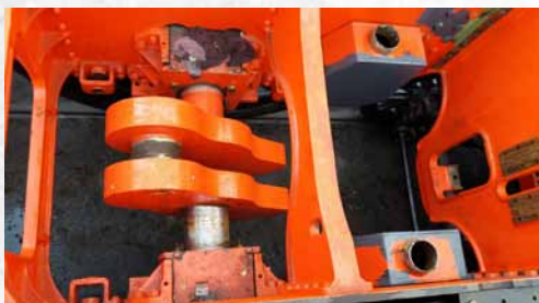
The Leading Sandboxes in position in the locomotive chassis.
