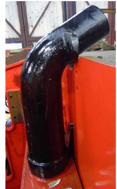
The Leading Sandboxes in position.
