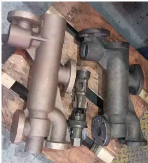
Injector body casting alongside an original injector.
