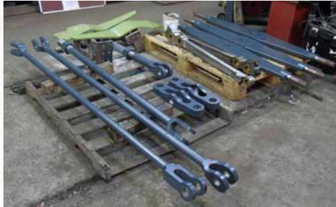
The Brake parts in undercoat. The two polished rods are the Outside Combination Levers formally fitted to Jubilee Class Achillies.
