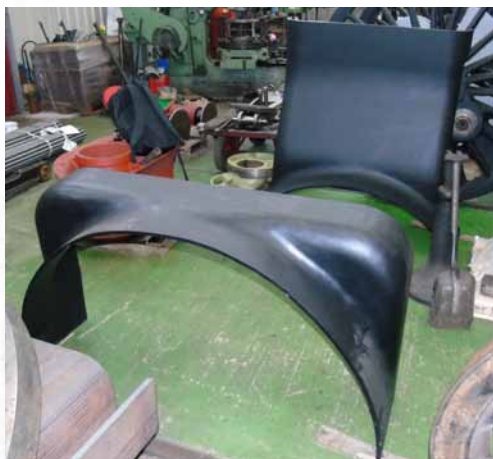
The two sections of the Throatplate at Tyseley Locomotives Works. In the foreground the Top section and behind the Bottom section standing upside down.
