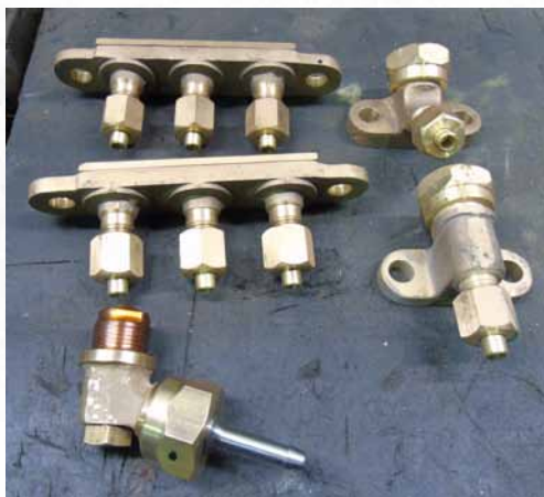
Another selection of fittings including for the Driving Axlebox Non Return Valves, bottom left.
