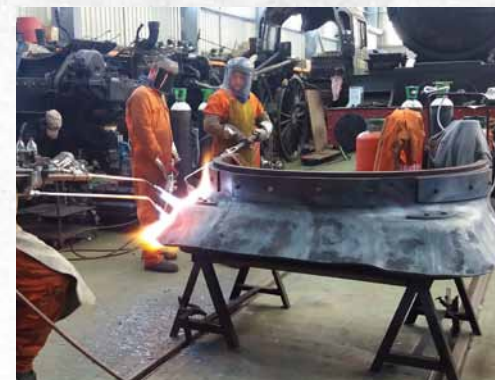
Throatplate Top 2 Heating another section of plate before hammering can begin.
