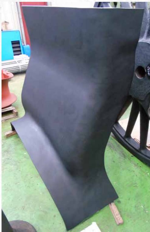
A side view of the Throatplate showing the 11/16" step below the Barrel flange at Tyseley Locomotives Works.
