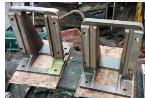
The Valve Guide Brackets being prepared for painting at Llangollen.
