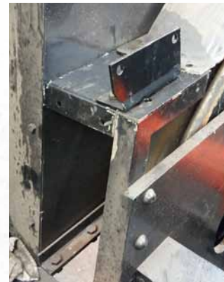
Left Hand Trailing Axle Guide Oil Box Bracket trial fitted to the locomotive chassis.
