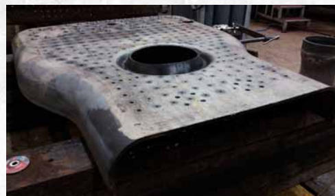
The Outer Firebox Doorplate undergoing drilling at LNWR, Crewe.
