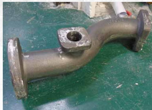
The casting for the Right Hand Main Steam Pipe at Premier Patterns. The square flange seen is the mounting for the Snifting Valve.
