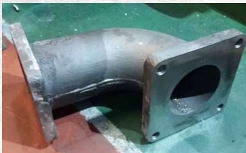
The Inside Exhaust Pipe after machining.
