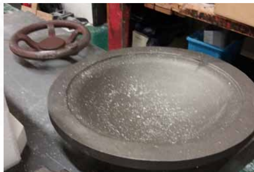
The Dome Cover casting and Reverser Wheel casting at Premier Patterns.
