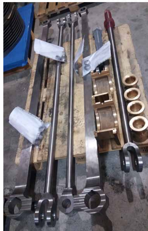
A selection of parts recently completed at CMS, including the two Outside Eccentric Rods and Brake Gear Pull Rods.
