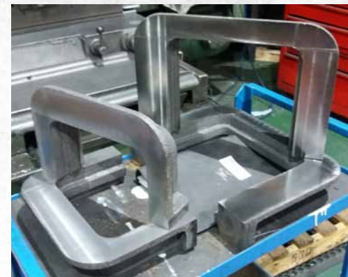
The Exhaust Seals during machining at Harco Engineering.
