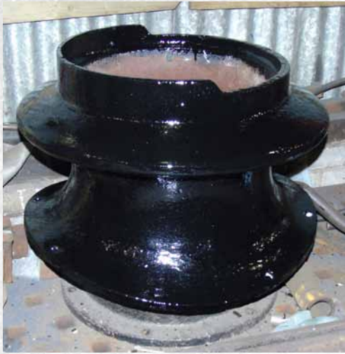
The repaired chimney from No. 5539 E. C. Trench.
