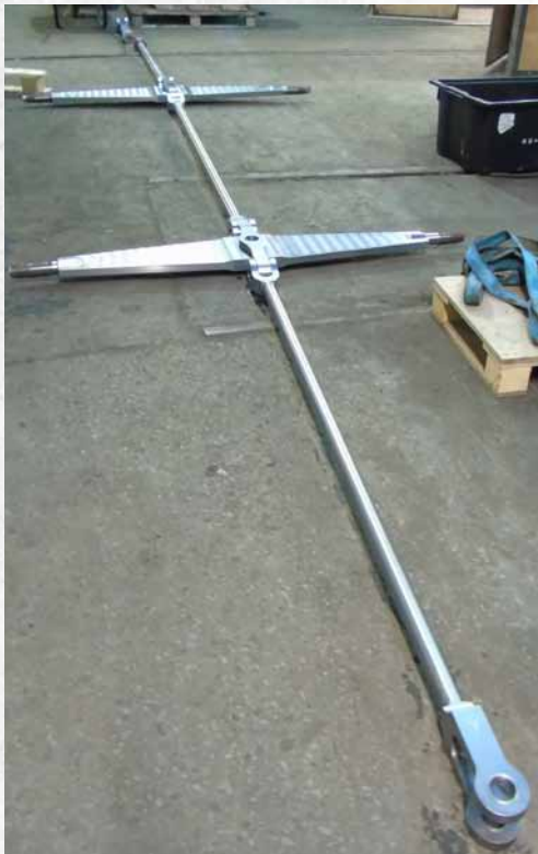
The Locomotive Brake Gear laid out on the floor at Llangollen Works. The third Cross Beam should be in the Pull Rod clevis in the foreground.
