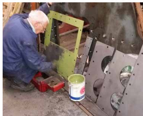
David Hughes painting some of the Smokebox Floor Plate at Llangollen Works.
