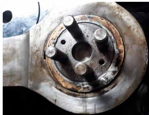
The left hand Trailing Crank Pin after removal of the Speedo Drive Crank showing excess white metal on the end of the bearing not removed. Also, the two Drive Dowels have not been fitted. PHOTO: KEVIN WEST
