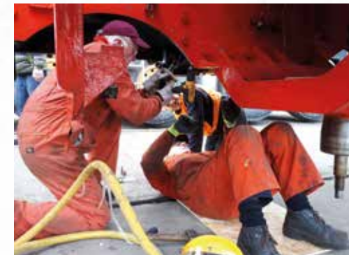
Gerry and Brian working on the cylinder cladding fixing holes. PHOTO: KEVIN WEST
