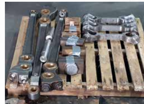
Above: A selection on Motion parts following removal from the locomotive. The three Combination Levers can be seen, the far left being the new Inside Lever and the original Outside Levers which are to be replaced.
