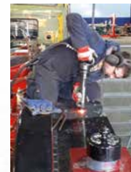
Andy from HBSS riveting the platforms. PHOTO: KEVIN WEST
