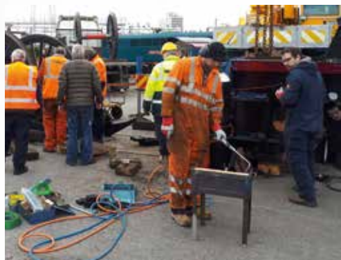
HBSS start work on riveting the Drag Box whilst the Axleboxes are removed from the Centre Driving Wheels.. PHOTO: KEVIN WEST
