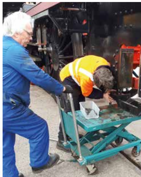
Steve Blackburn and Nigel Day refit one of the Horn Ties. PHOTO: KEVIN WEST
