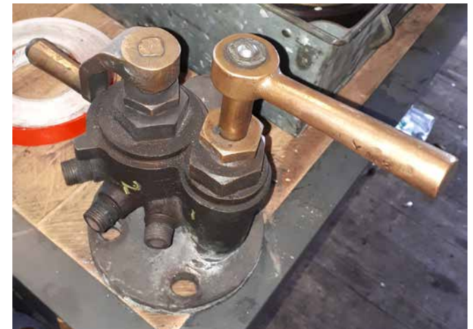
Blower & Sanding Valve from Crab No. 13065 at East Lancs Railway.
