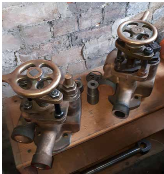
The Injector Water Valves and Clack Boxes from Crab No. 13065 at East Lancs Railway.
