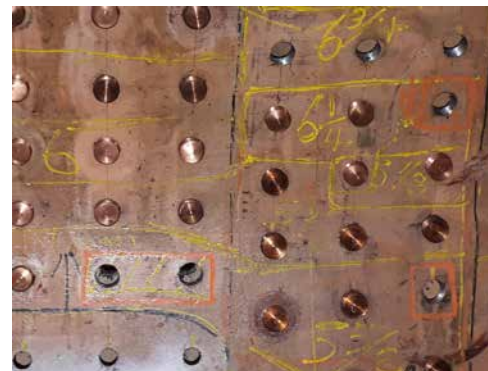
A view of the Firebox side showing the plate marked up with the correct length of stays required. Photo - Kevin West
