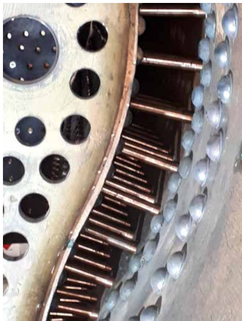
A view of the left side of the Firebox with most of the Stays installed.
