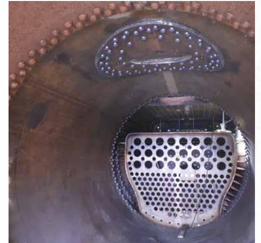
An interior view of the boiler. The Inner Firebox can be seen at the far end with the Dome doubling plate riveted into the top of the barrel.
