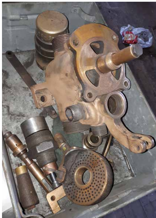
The Drivers Brake Valve from Crab No. 13065 at East Lancs Railway.
