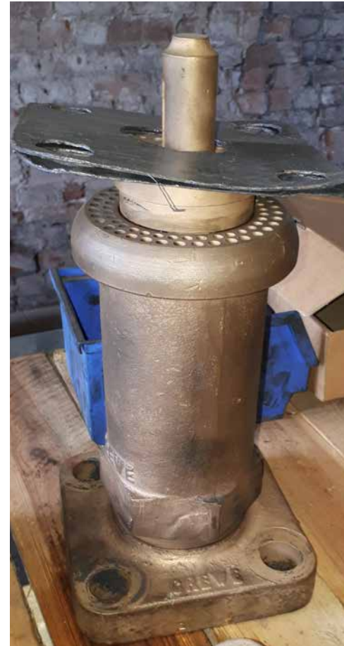
A Safety Valve from Crab No. 13065 at East Lancs Railway.
