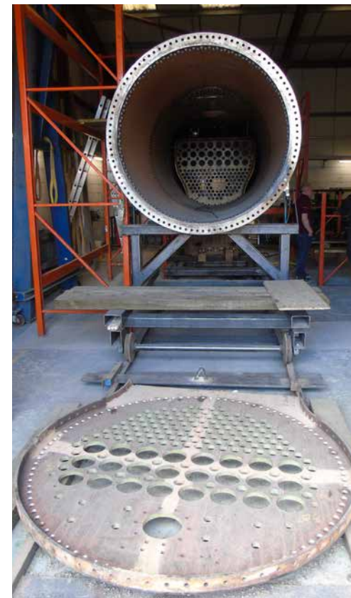
A view of the boiler with the Tubeplate in the foreground.
