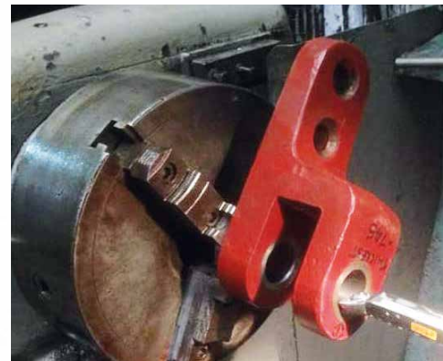
One of the Spring Link Brackets being bored after a new bearing had been pressed in..
