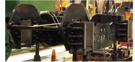
Bogie Frame at West Shed, 4th February 2020.
