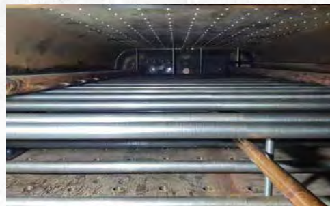
Transverse Stays inside the Firebox. Photo: HBSS
