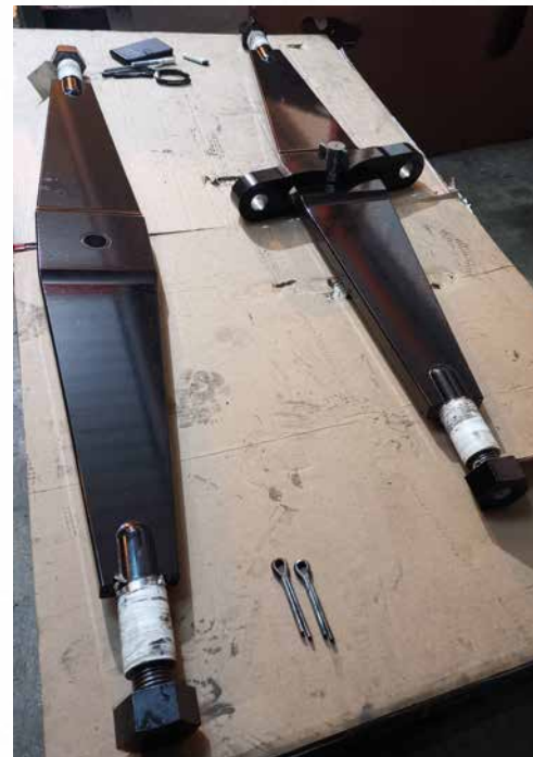
Repainted Brake Cross Beams. Photo: Gavin Shell
