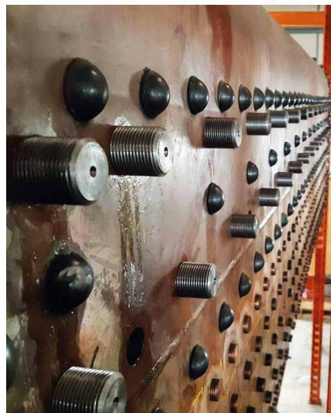
Left hand side of the Firebox showing the threaded ends of the Transverse Stays. Photo: HBSS
