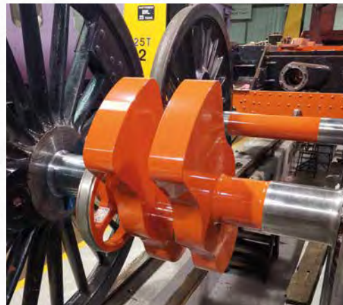
Crank Axle following completion of painting. Photo: Gavin Shell
