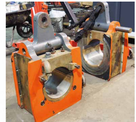
Driving Axleboxes await attention at West Shed. 4th February 2020. Photo: John Hastings-Thompson
