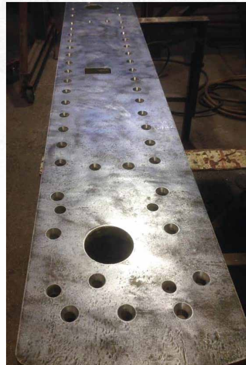
Tender Buffer Beam following drilling.
