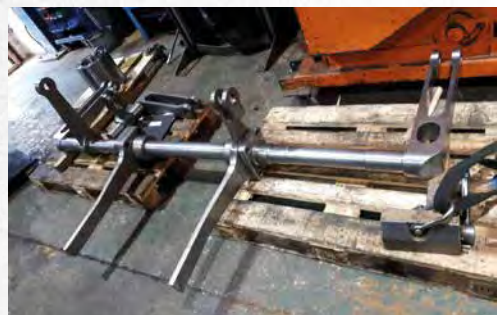
The Reverser Shaft assembly at Roach Engineering, January 2020. Photo: Kevin West
