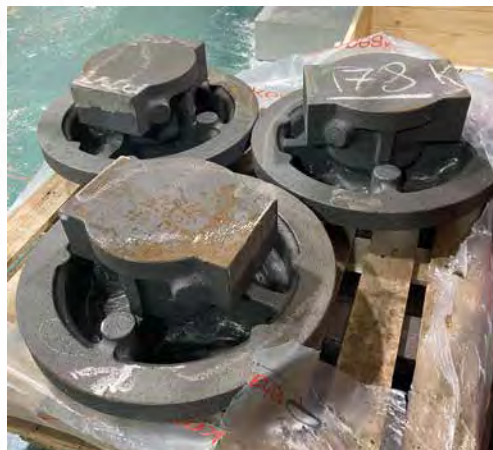
Rear Cylinder Cover castings. Photo: Premier Patterns
