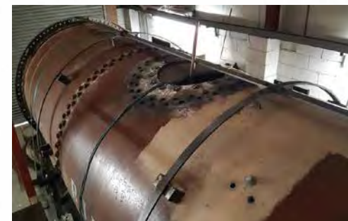
Left hand side of the Firebox showing the threaded ends of the Transverse Stays. Photo: HBSS
