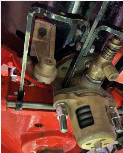
View underneath the Inside Cylinder showing Cylinder Relief Valve, Drain Cock and Operating Gear trial-fitted. West Shed, November 2019. Photo: Andy Collinson
