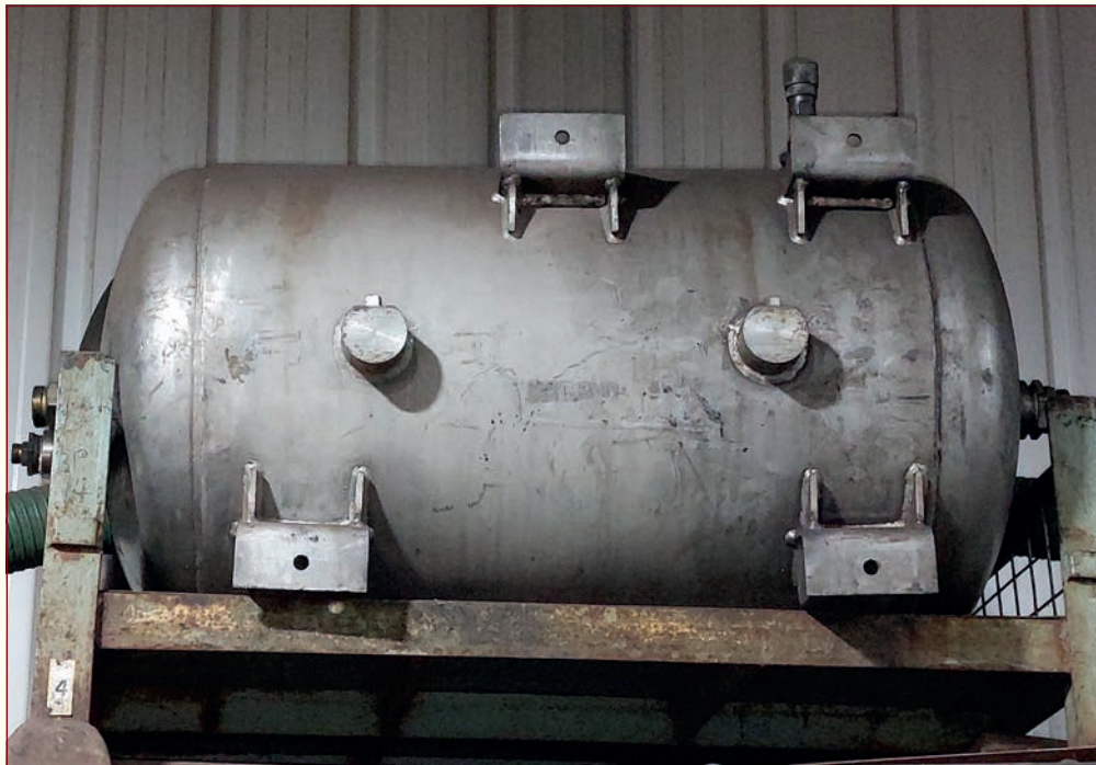
Air Tank to be fitted under the tender of 5551. PHOTO: KEVIN WEST
