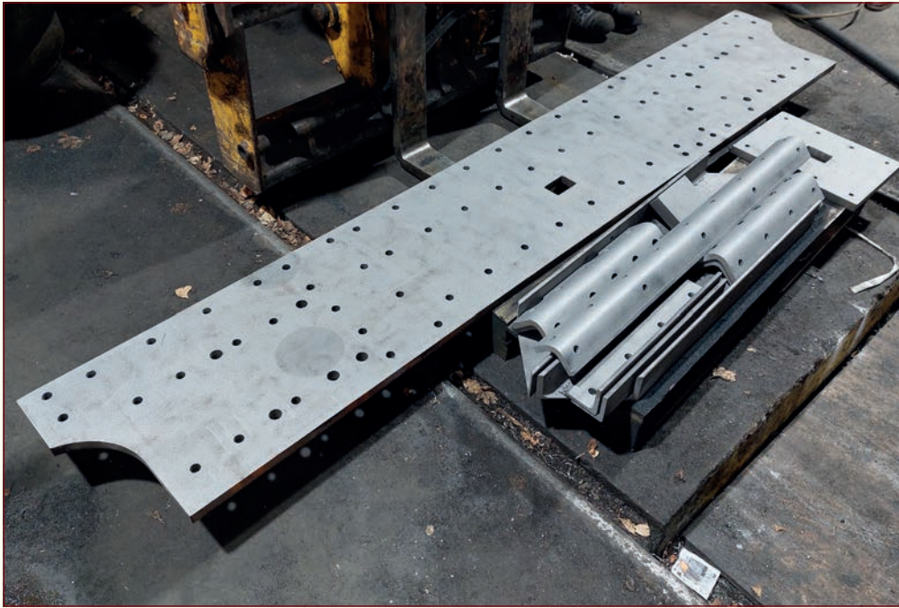
Above: The new Front Buffer Beam and Mounting Brackets.
