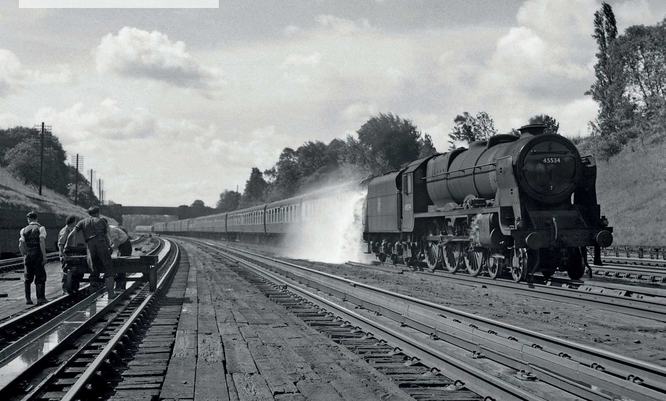
Rebuilt Patriot 4-6-0 No. 45534 E. Tootal Broadhurst takes water from Bushey troughs with a Euston to Liverpool express on 12th August 1956. PHOTO: C. R. L. COLES/RAIL ARCHIVE STEPHENSON
