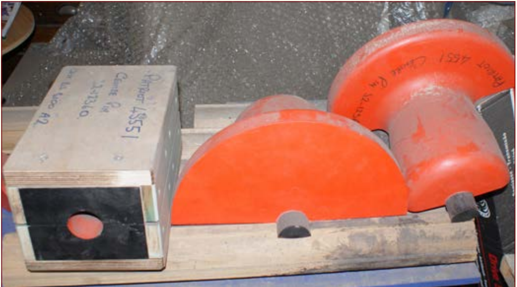
Above: The pattern pieces for the Patriot Bogie Centre Pin. The Core Box on the left and the two body pieces on the right.
