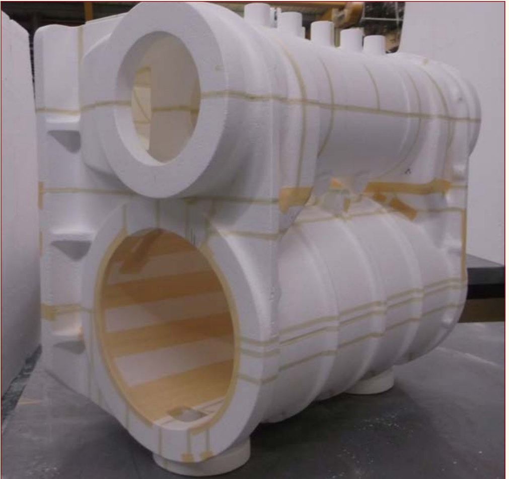
Below: The completed pattern for one of 5551's Outside Cylinders.
