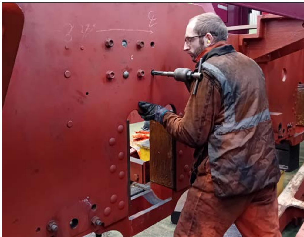
Above: Reaming holes for Rivets before fitting of Frame Stretcher.
