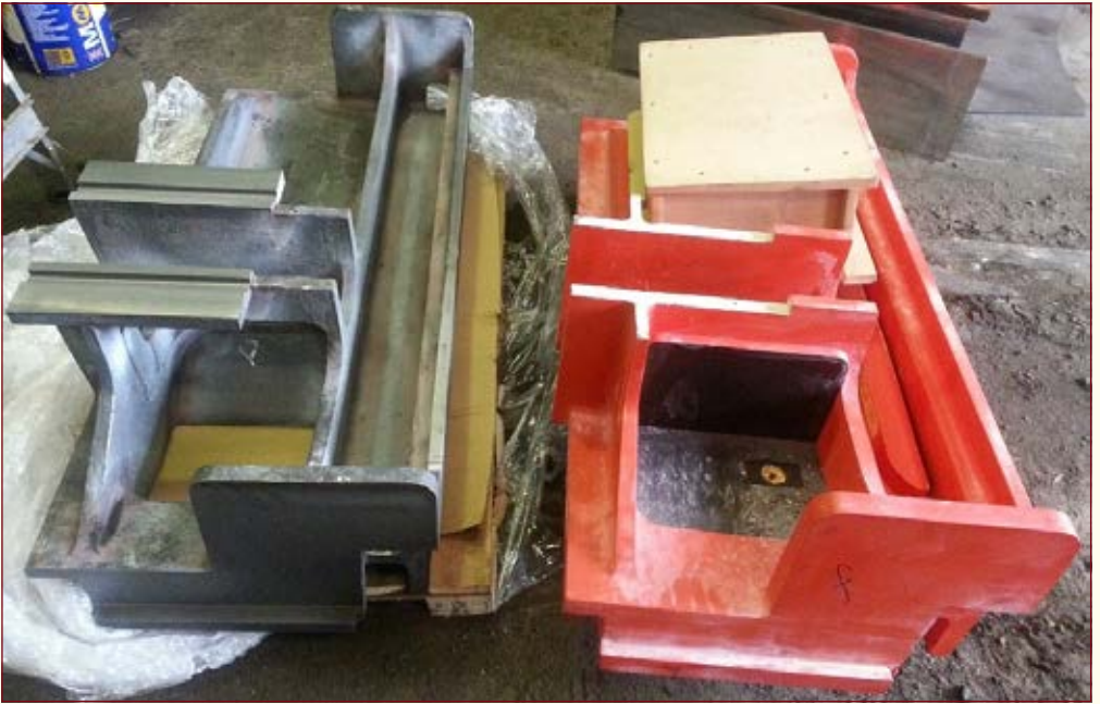
Above: The casting and pattern for one of 5551's Stretchers.
