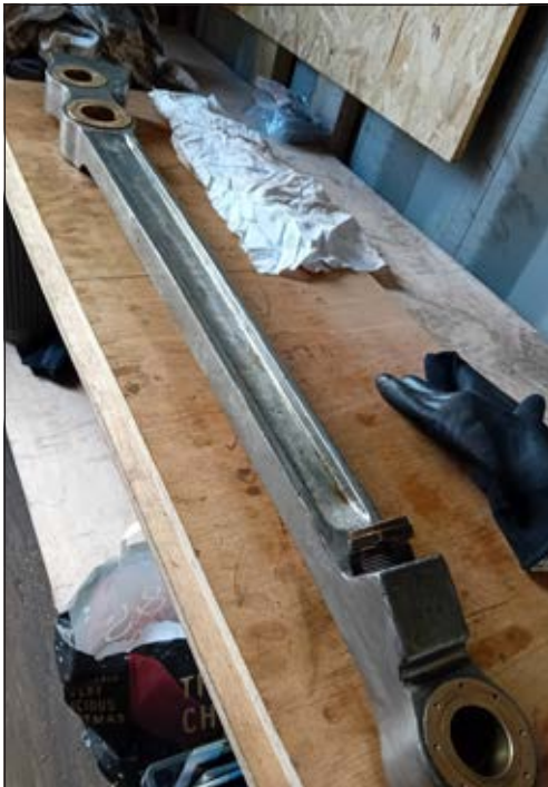
Bottom Right: A set of Outside Valve Rod Die Block Slide components, following preparation for fitting.
