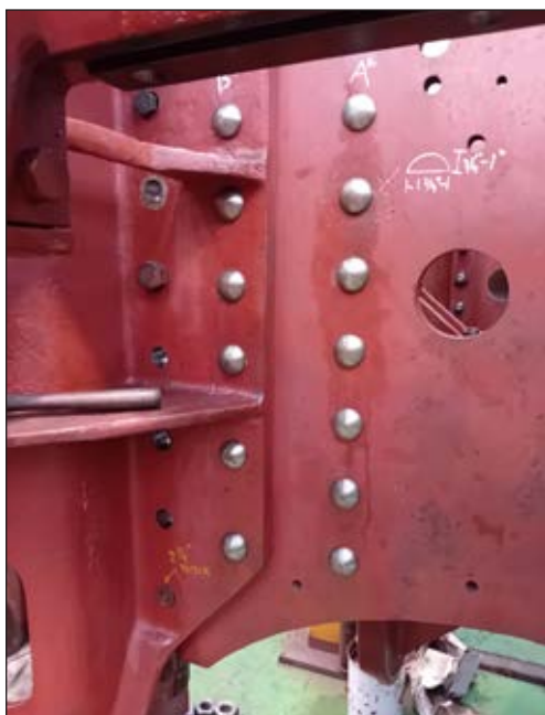
Above: Reaming holes for Rivets before fitting of Frame Stretcher.
