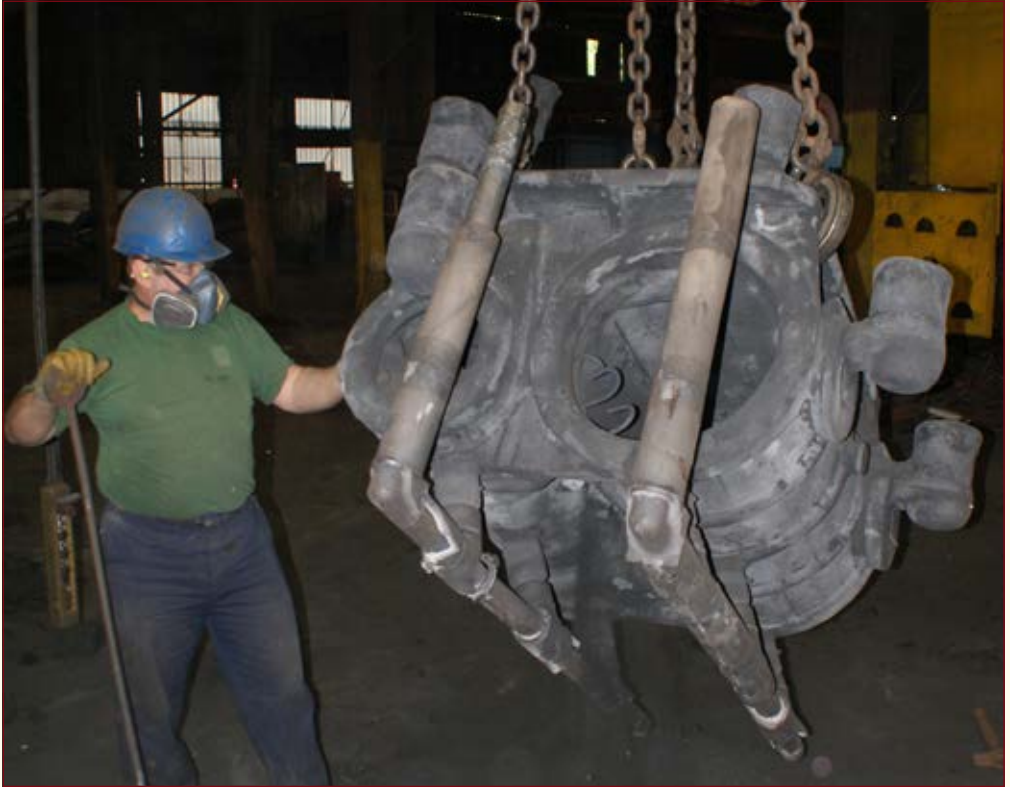
Above: Outside Cylinder casting after cooling and knocking out of the mould. The Runners and Risers can be seen before they are cut off from the casting.
