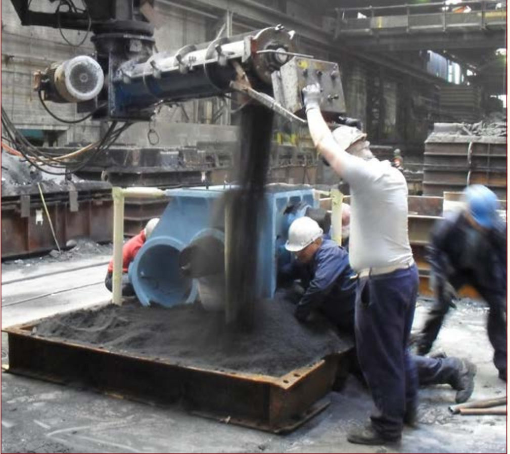
Above: The sand being delivered by overhead chute, while the foundry men compress the sand around the pattern.
