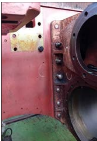
Above Left: Right Hand Outside Cylinder, showing the Fitted Bolts being installed.
