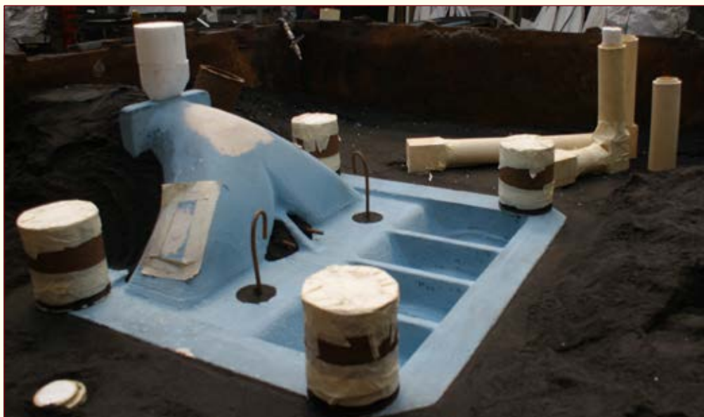
Above: The mould for an Outside Cylinder during build up, showing the risers and runners. The iron bars are reinforcements for the sand in internal areas of the casting. The rest of the mould will be filled with sand compressed down on top of the pattern.
