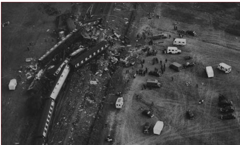
21ST SEPTEMBER 1951 • With the continuing effects of delayed maintenance following the war, when the expedient of swapping round the wheel and axle of the bogie of a locomotive met a length of track overdue for renewal, disaster ensued at Weedon. No. 6207 Princess Arthur of Connaught with the 8.20am 15-coach train from Liverpool to Euston, having passed through Stowe Tunnel south of Weedon, derailed. The rapid deceleration of the locomotive, as it fell on one side, caused seven of the following coaches to concertina into a zigzag pattern. The driver and 14 passengers died in the ensuing mêlée. Here several ambulances and fire engines, together with Police and other cars, are in attendance with their crews attempting to rescue the injured and extract the dead. PHOTO: UNATTRIBUTED, AUTHOR'S COLLECTION
