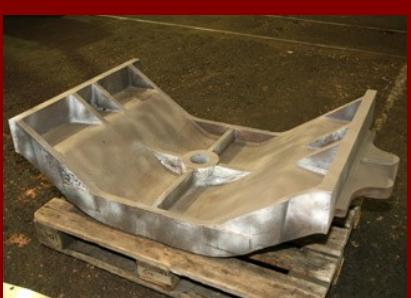
The nearly completed bogie bolster is seen at the Boro Foundry on 15<sup>th</sup> September 2010. Further machining was due to take place before being delivered to Llangollen for fitting on 'The Unknown Warrior'. Photo by Bob Sweet.
