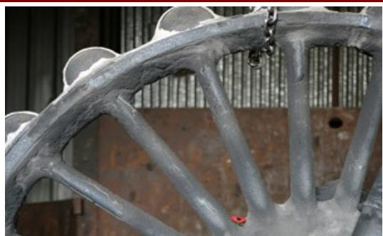
It would be two days before the fierce liquid heat would cool to a tarnished silver, and the mould would be cracked open to reveal the wheel within. Then the work started. The pouring risers had to be machined off and the wheel shot-blasted clean until it was a gleaming, gunmetal grey. Then it was whisked away for x-ray and heat treatment, whilst work began on the remaining five driving wheels.
